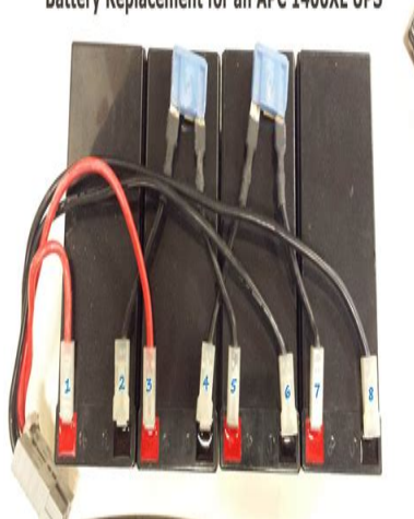
Battery Replacement for an APC 1400XL UPS
